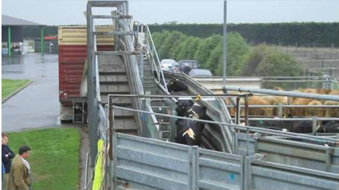
Figure 3: A single send and receive pair of antenna mounted above cattle at 2.6m height
