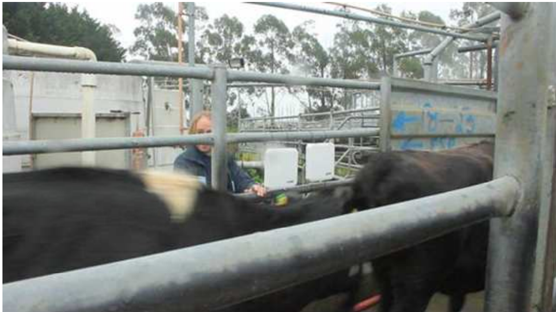
Figure 4: Moving the send-receive antenna pair to the side improved results; in practice send/receive antennas above and beside animals would perform better.
