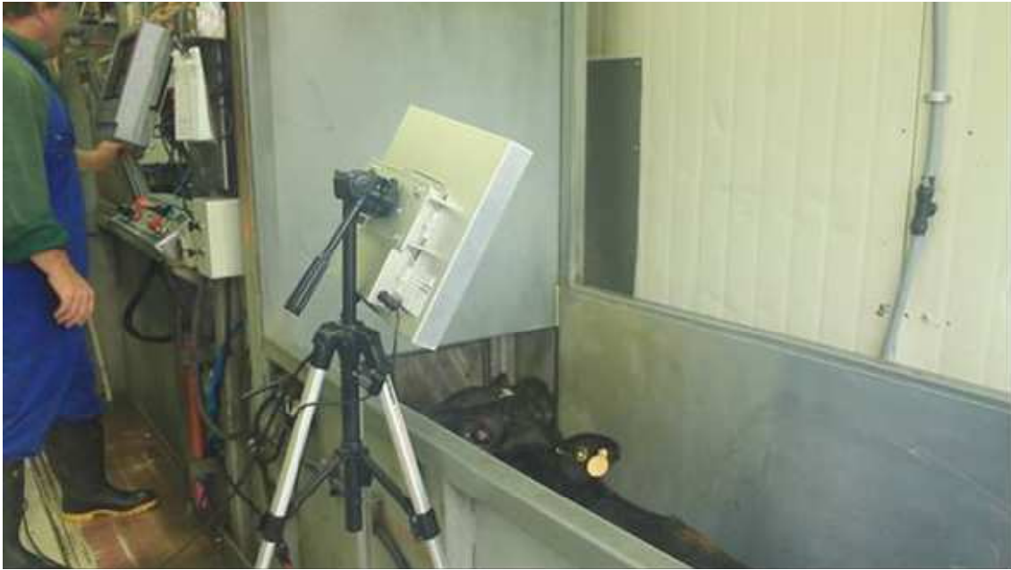
Figure 5: Reading individual cattle with an integrated reader at the stun box.
